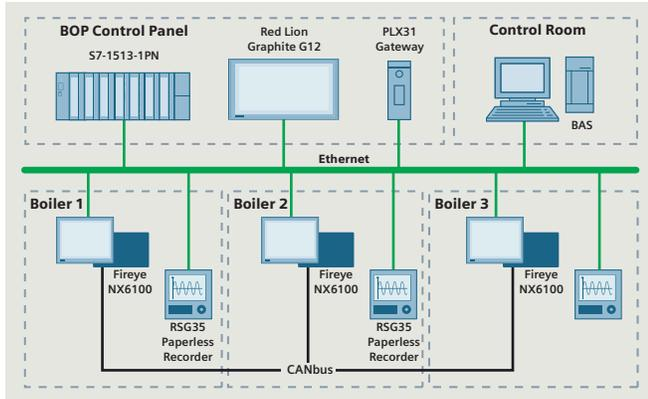
Figure 1. Upgraded architecture of boiler and BOP solution
