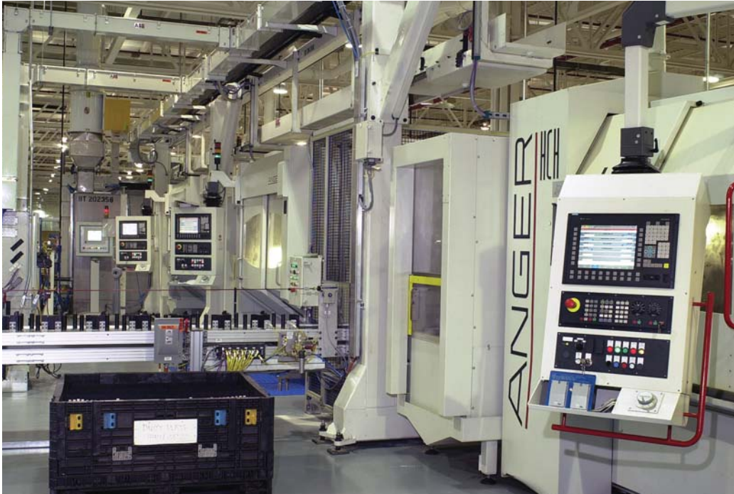
High-speed cutting machinery all feature easy operator interface, data screen call-up and programming capability
