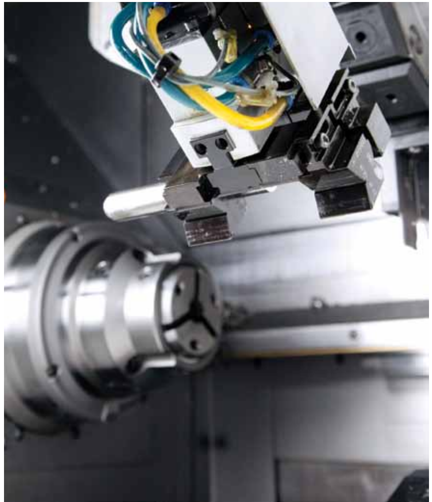
The INDEX C100 features automated remnant removal. The design has helped TFT increase revenues by eliminating the production delays caused by manual remnant stock removal cycles — typically not an option on lower-priced machines.
