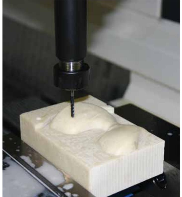
RenShape being machined on the DMG milling center
