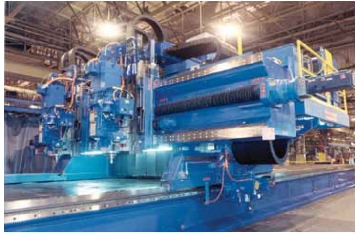
Cincinnati gantry mill produces long aero structures. This machine has been retrofit several times
