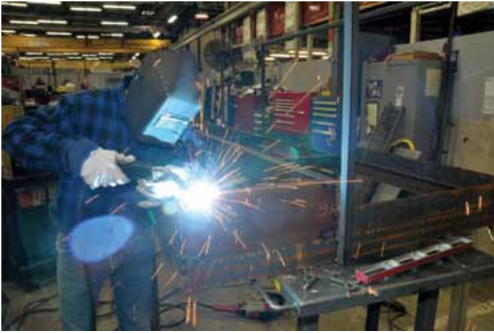
Spirit welding shop where various support structures are fabricated
