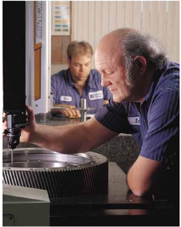
Touch probe inspection of gear diameters
