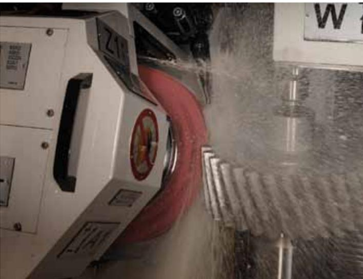
Reishauer RZ400 gear grinding machine with Siemens Sinumerik 840D CNC. Machine is show grinding gear teeth.
