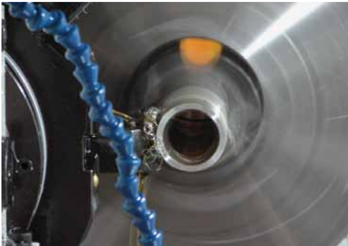
OD turning at Continental Machine produces a variety of prototype and production parts
