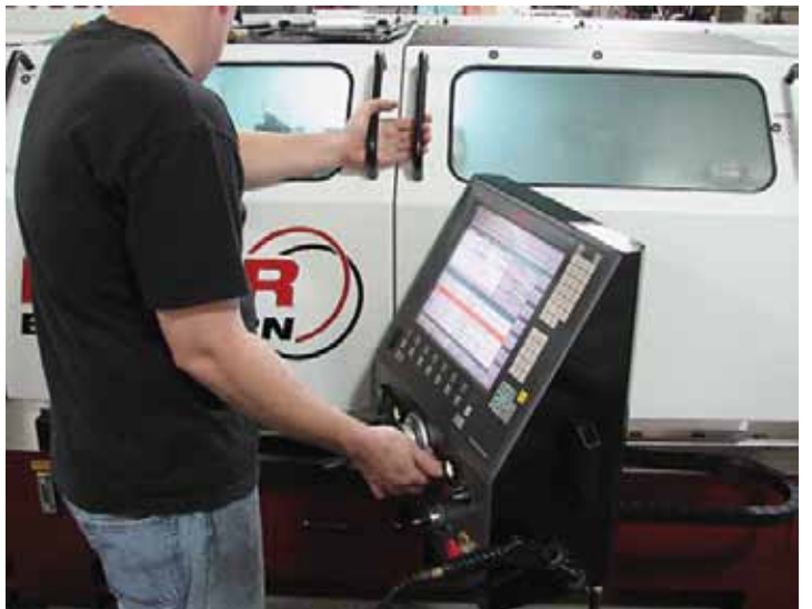
Siemens SINUMERIK 840D sl CNC onboard the Fryer Easy Turn combination lathe
