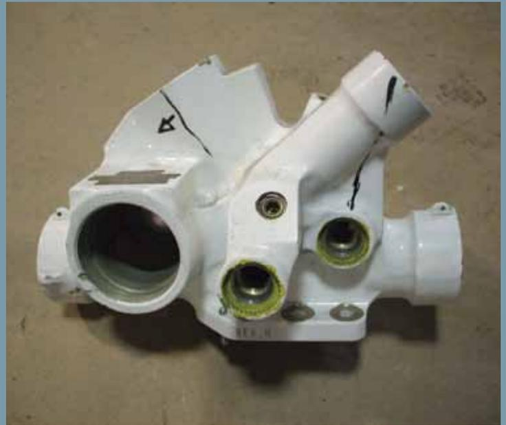
Five-axis machining reduced the number of setups from 23 to 4 to produce this part
