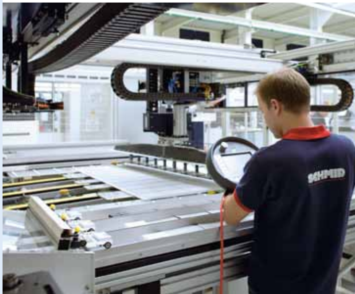
A Schmid employee at the Mobile Panel for teaching positions during active SLS inside the machine
