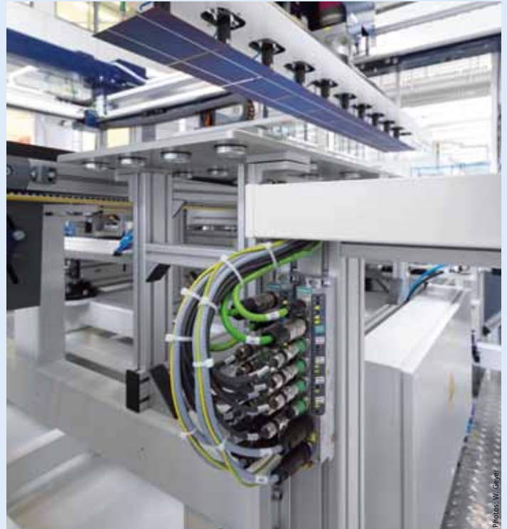
Simatic ET200eco for connecting the distributed peripherals, rotary grippers for the strings
