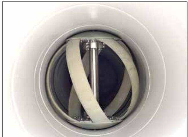
*Siemens motors are powered by the turbulent flow of the water through the municipal water line. The energy is captured and transmitted to the PGE grid for powering the local community.*
