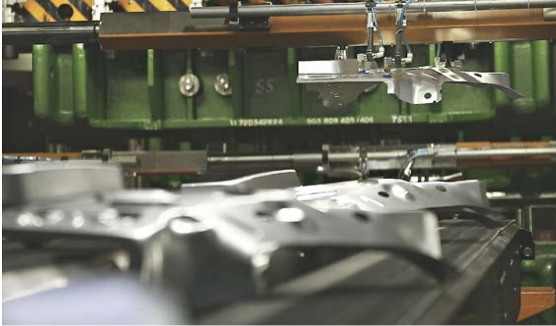
At Volkswagen in Wolfsburg, vibration sensors in press line 400 monitor the status of the main motor's bearings
