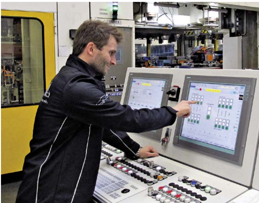
The Siplus CMS X-Tools software analyzes, visualizes, and archives the measurement data and provides corresponding indications on the condition of machines and plants
