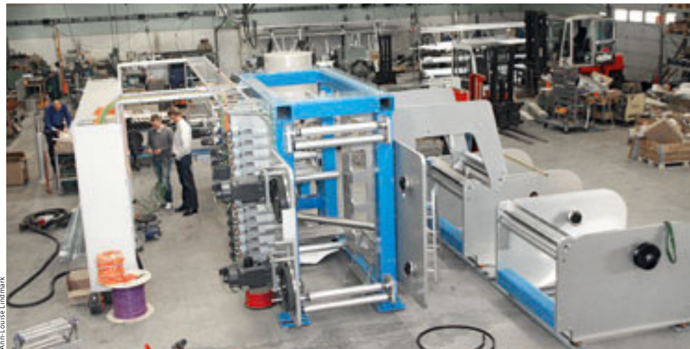
A view of the Trancel Restatic workshop showing a machine for producing environmentally friendly plastic bags from biodegradable material
