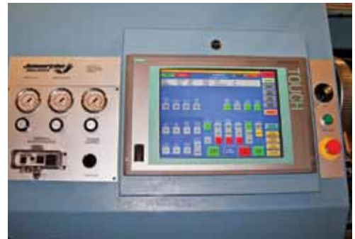
Siemens controls onboard this Jennerjahn JLS-120 slitter rewinder, a specially modified machine sold to a building products customer in Australia, who required components to suit a 415VAC, three-phase electrical power supply. The machine also has three additional ancillary axes of motion. The HMI, PLC, drives package and Profibus DP communications network were all provided by Siemens through its local distributor.
