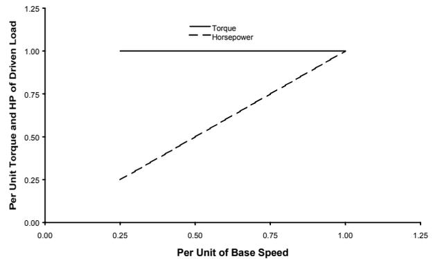
Fig. 2. Constant Torque Load Curve
