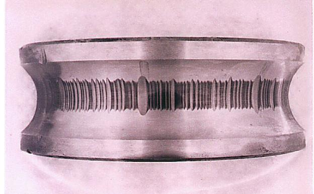
Fig. 7. Anti-Friction Bearing Inner Race With Severe Fluting
