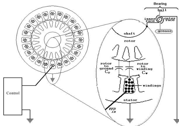
Fig. 8. Path of Common Mode Voltage the Stator Windings to Ground
