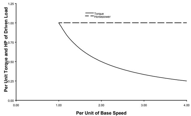
Fig. 3. Constant Horsepower Load Curve
