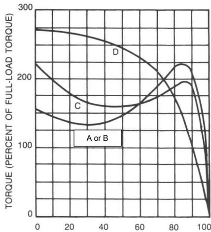
Fig. 5. NEMA MG1 Load Designs for Induction Motors Operating on Sine wave power
