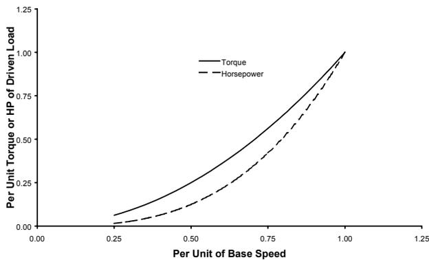
Fig. 1. Variable Torque Load Curve
