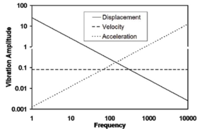
Figure 14 Comparison of vibration amplitudes Expressed in acceleration, velocity, and displacement
