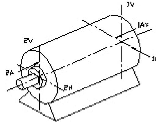
Figure 15 Vibration Measurement Positions
