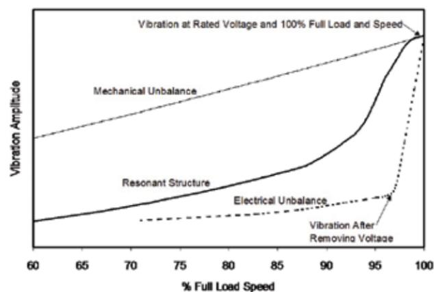
Figure 16 Vibration After Power is Removed
