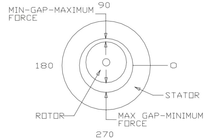
**Figure 4 Unsymmetrical Air Gap Around Rotor**
