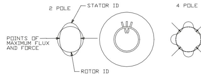
**Figure 3 Electromechanical Force on 2 & 4 Pole Motors**
