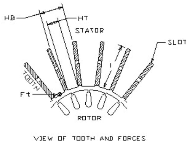
Figure 10 Stator Tooth Forces
