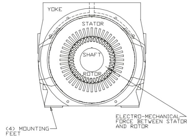
**Figure 1 Stator and rotor**
