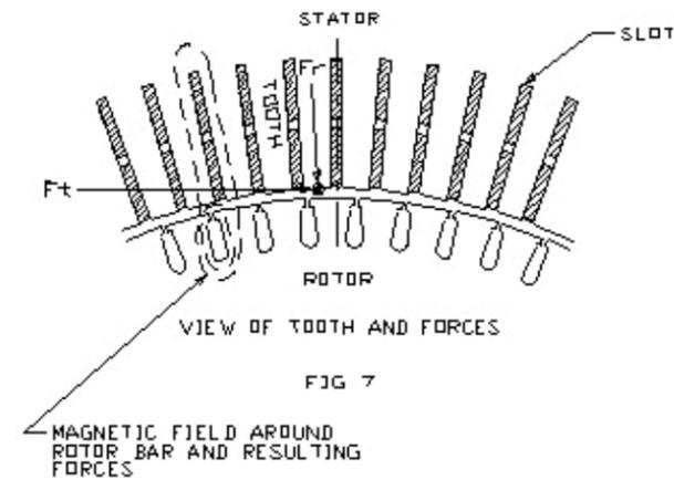
Figure 7 Magnetic Field around Rotor Bar and Resulting Force on Stator Teeth
