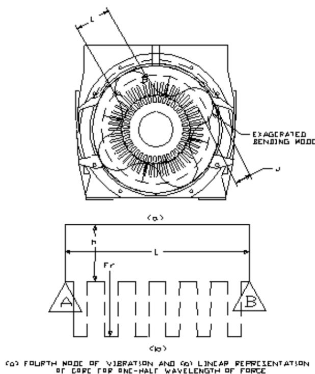
Figure 9 a) Fourth Mode of Vibration
