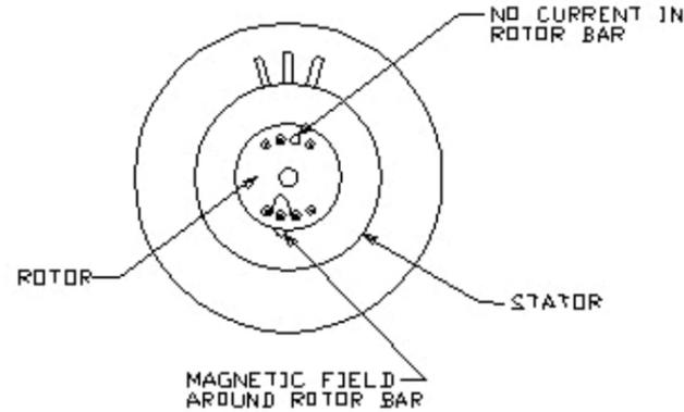
Figure 6 Rotor with Broken Rotor Bar
