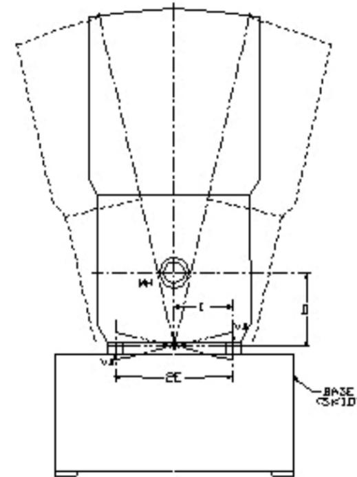
Figure 12 Rocking Mode due to Weak Base
