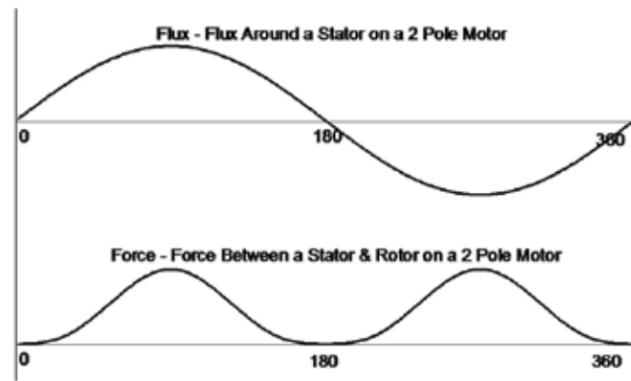
**Figure 2 One Period Flux Wave & Magnetic Force Wave**
