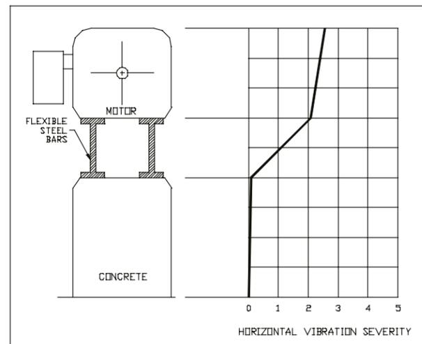
Figure 11 Plot of Vibration (in mils) Vs. Base/Motor Position
