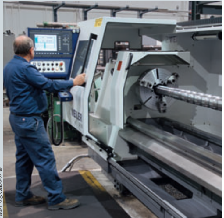
RER plant manager Bob Merriman at the Weiler E70 CNC lathe equipped with Sinumerik 840D
