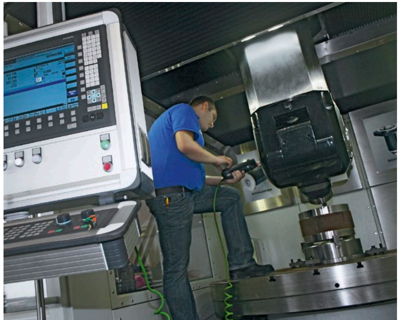
The Sinumerik 840D sl CNC enables changeover from one machining head to another in less than one minute
