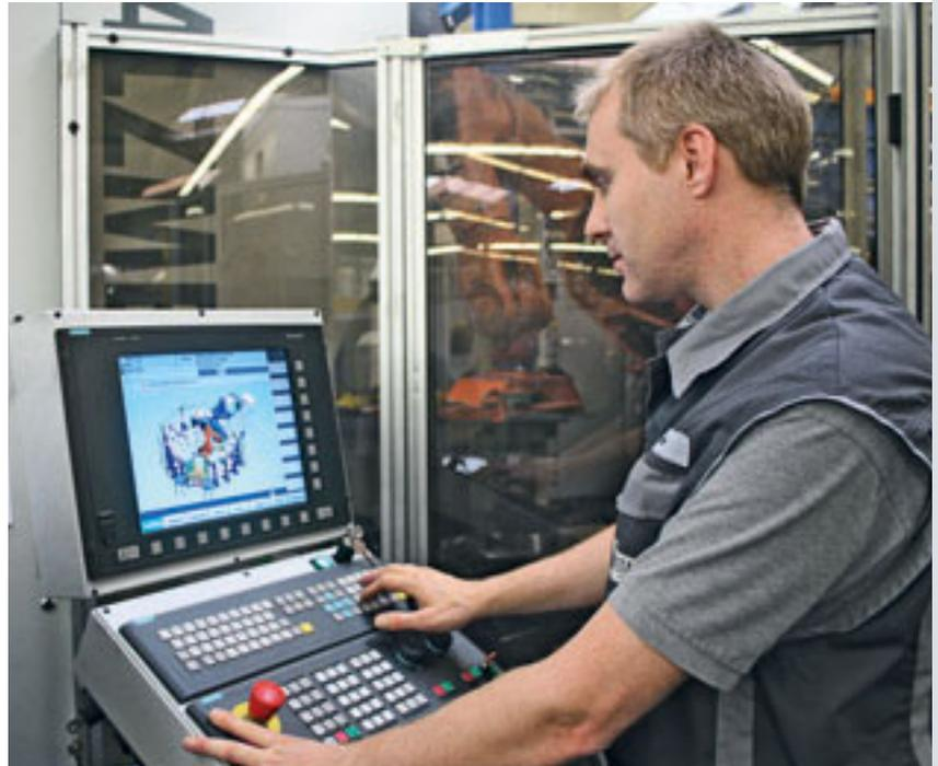
The Sinumerik Operate operator interface is very similar to that of a PC; during set-up, the operator is supported by graphical displays and animated images
