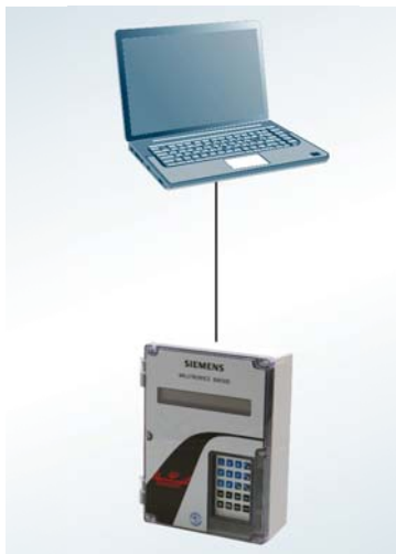
Figure 3: Controller/monitor to one device, in this case, Milltronics BW500 weighing integrators from Siemens.
