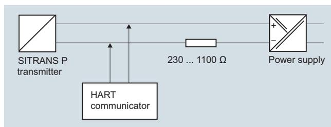
Communication between a HART Communicator and a pressure transmitter
