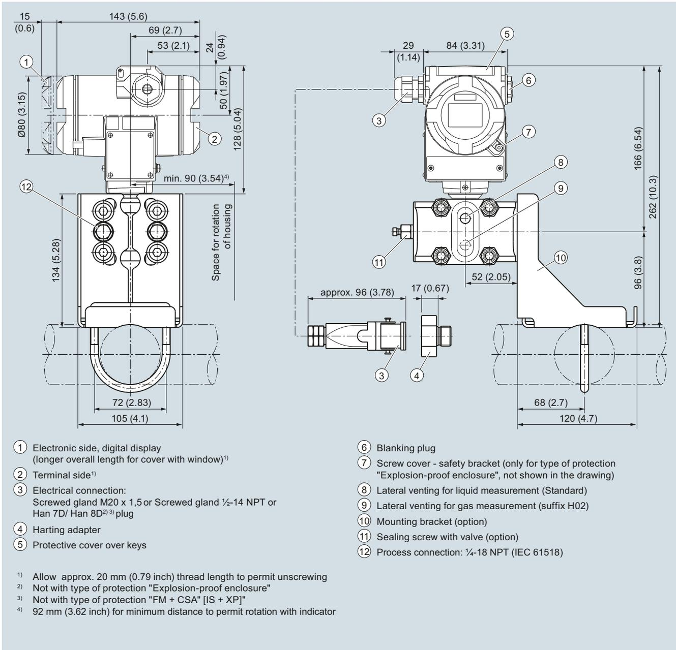
SITRANS P310 pressure transmitters for differential pressure and flow, dimensions in mm (inch)
