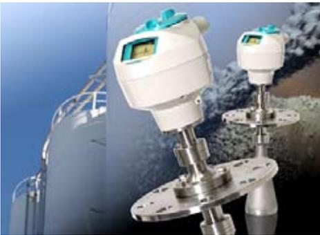
A SITRANS LR260 unit was installed on each of three silos to provide product level indications. A separate RD-200 unit (a universal input, panel-mount remote digital display for process instrumentation) was used to power each unit and provide display of level. Each remote RD-200 display unit is mounted on a panel located in the dispatch/control room. Before a
