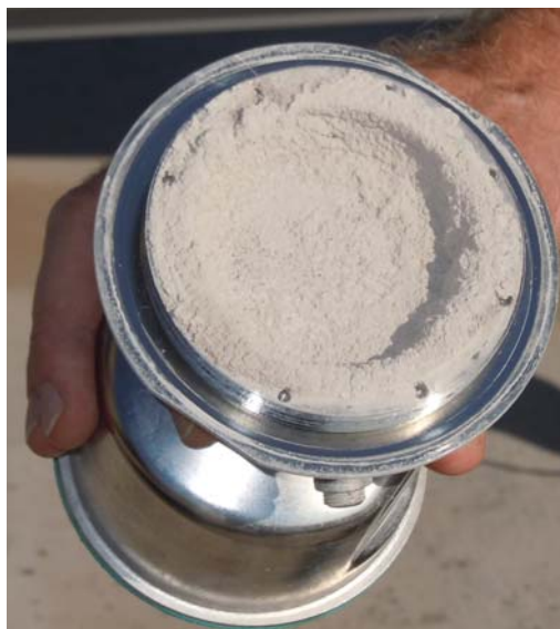
Figure 3 (left) and Figure 4 (right): SITRANS LR560's highly durable polyetheramide lens antenna (left) can tolerate significant buildup, such as in this photo (right), where it has been coated with finished cement powder.
