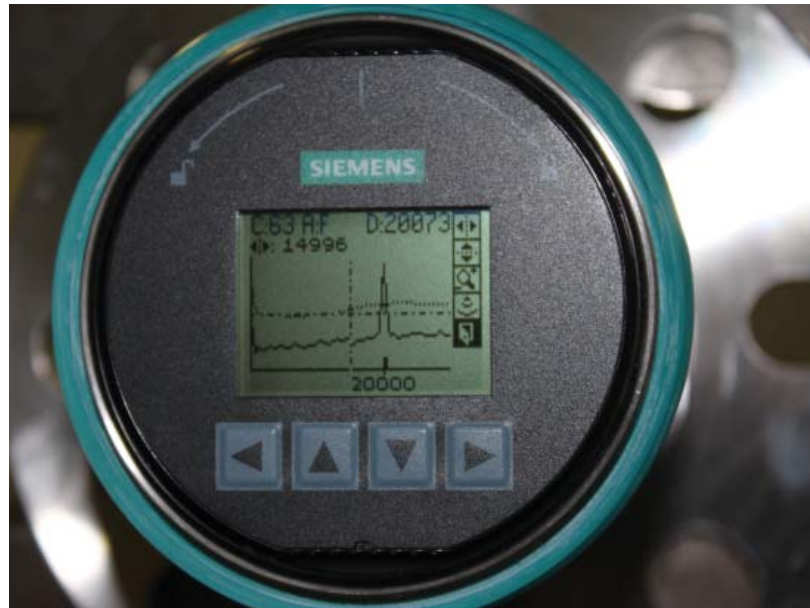
The company's operators can read their silo's echo profile on SITRANS LR560's Local Display Interface (LDI).
