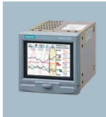
The SIREC D200 recorder has a 5" color display.
