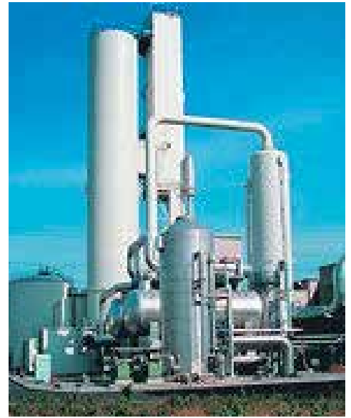
Fig. 2: Typical air separation plant
