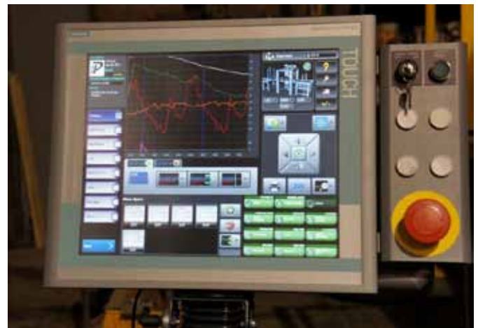
Figure 3, screen shot: This totally-enclosed 19-inch touch screen panel has been customized with CTI's software application written to run on a Linux-based industrial PC.
