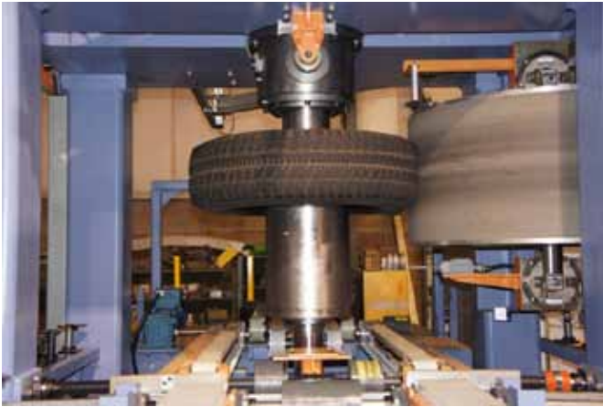
Figure 5, tire testing: During tire uniformity testing, the tire is rotated against a loadwheel and measured for force variations.
