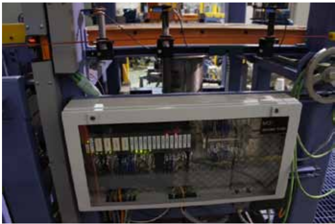
Figure 4, distributed I/O: Distributed I/O simplifies machine wiring, reduces debug and commissioning time, and reduces susceptibility to electrical noise.
