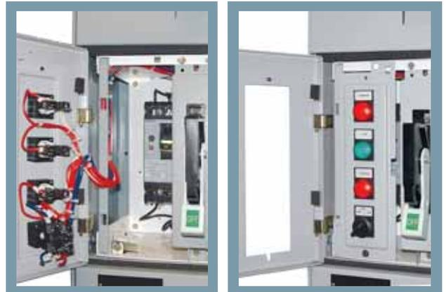
Unit Terminal Blocks are conveniently mounted up front on a swing-out side barrier for ease in wiring and inspections.
