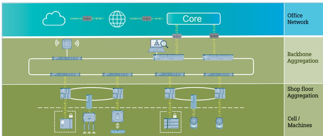
Connecting the IT and OT networks, with their different requirements, can be accomplished by starting with a defined backbone for the industrial side. The Cell/Machine and Shop-floor Aggregation levels are in production scope. The Backbone Aggregation level is still an integral part of the production scope but aligned with IT in regard to the interface.
