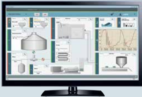
Web-based operator control and monitoring with SIMATIC WinCC WebNavigator
