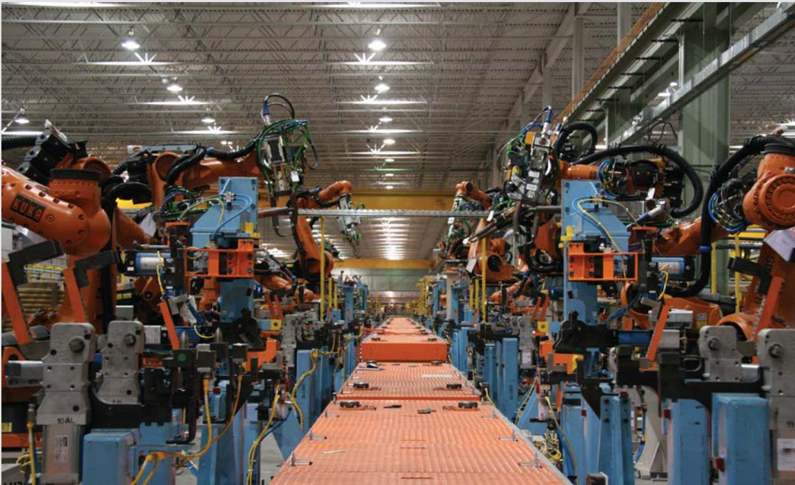
Utilizing robots, adhesives are applied and body panel components are welded inline.
