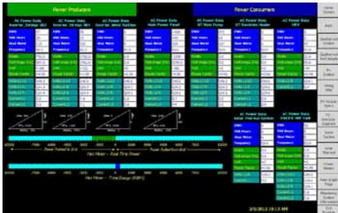
Screen capture from 12" comfort panel showing all power information for entire home
