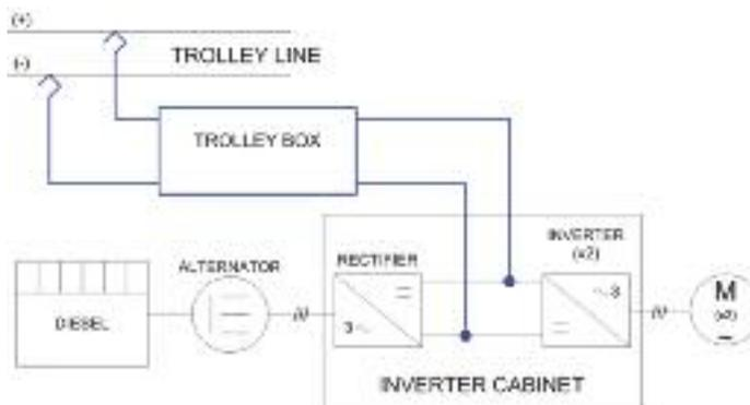
Figure 1. Diagram of typical diesel/electric haul truck with trolley assist option
