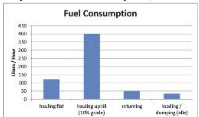
Figure 2. Typical haul truck fuel consumption during various phases of hauling cycle
