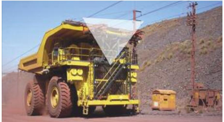
the pantograph and/or the overhead lines. Damage to the pantograph takes the truck out of operation, at least out of trolley operation. Damage to the overhead lines takes the entire trolley fleet out of operation.
