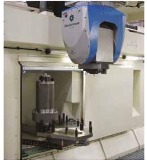
Left: Zimmermann FZ42 portal milling machine with five-axis, five-sided cutting capability
