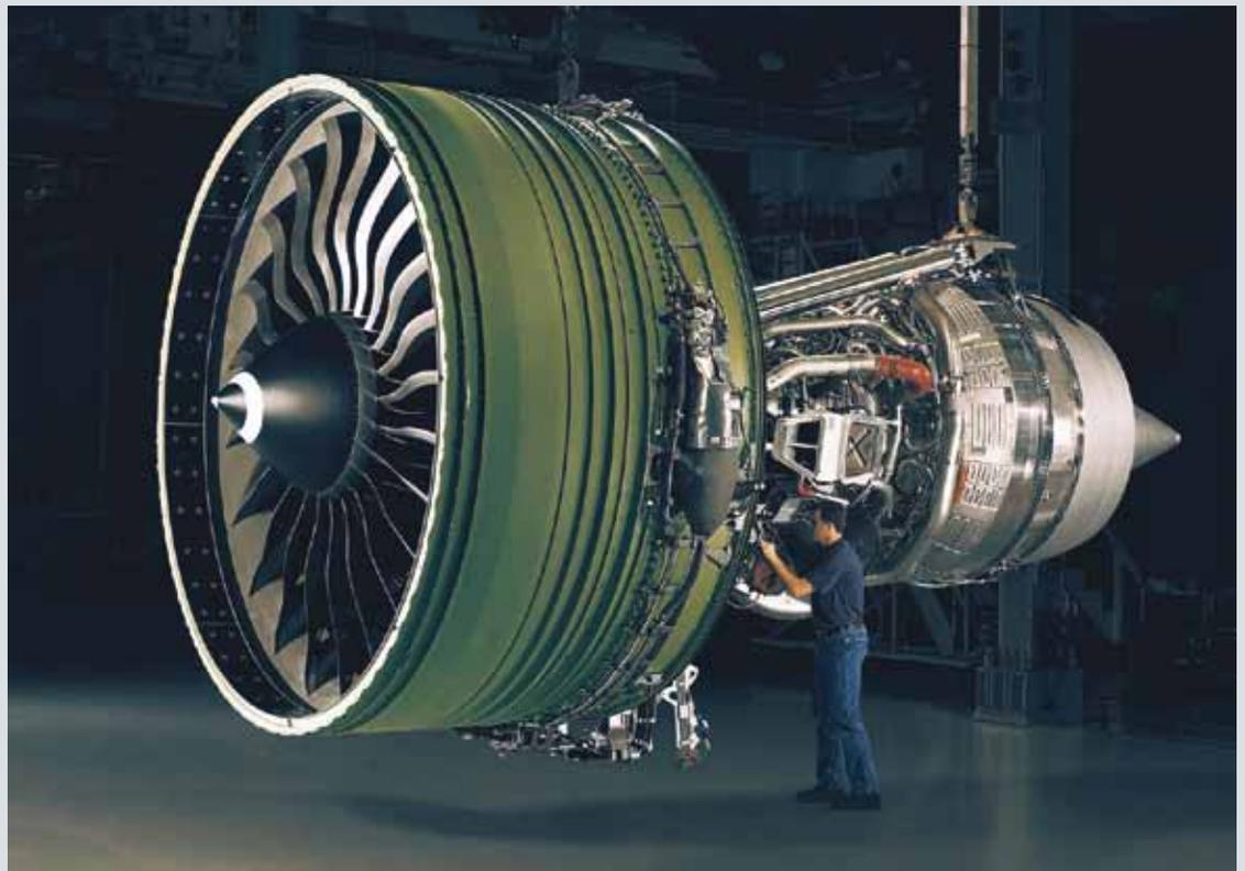
GE90 engine; Volvo Aero Connecticut made the fan casing, currently the largest of its kind at 3.5m (11.5 foot) diameter
