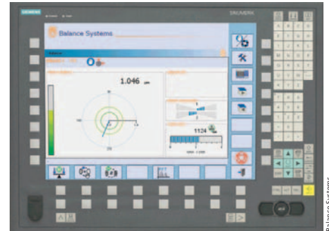
Balance Systems developed a measurement and control system for grinding machines for use on the Sinumerik
