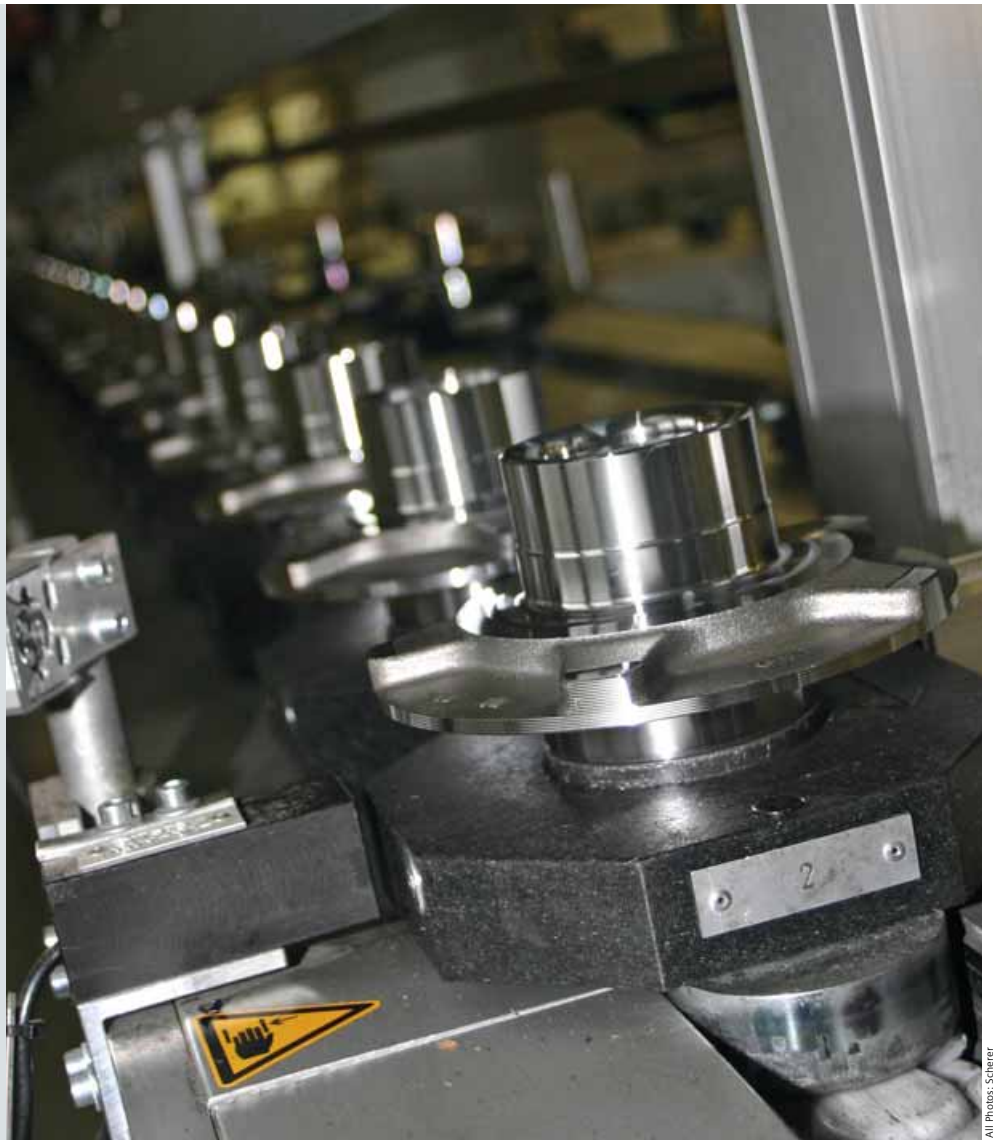
Audi wheel hubs on the way to final hard machining
