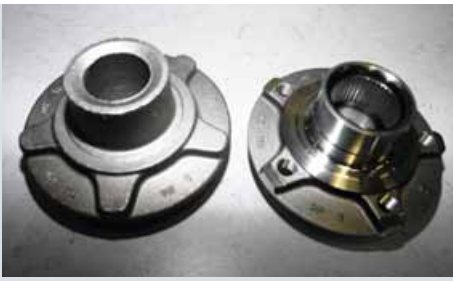
Before and after: wheel hubs machined on Scherer Feinbau VDZ 120 DS vertical centers with Sinumerik 840 sl CNC
