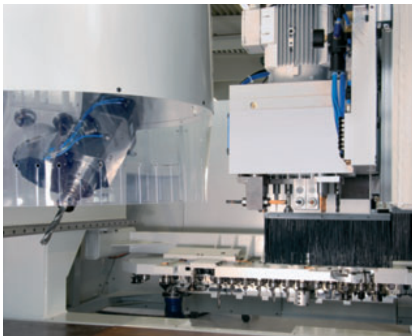
The swivel unit of the Vision machine enables precise machining from all sides
