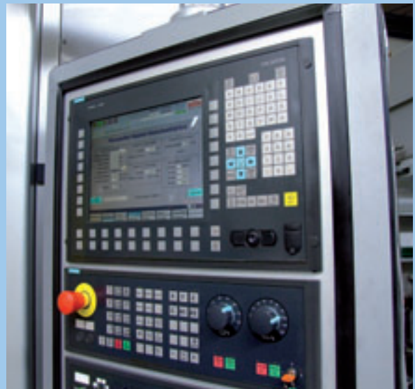
Eldec has taken the openness of the Sinumerik 840D and installed its own, easily configured user interface
