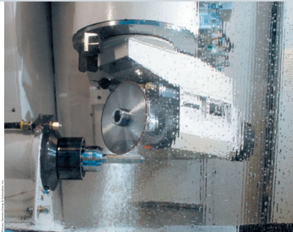
The Schütte WU 305 Linear universal CNC cutter grinder performs milling, grinding, belt sanding and polishing all in one operation
