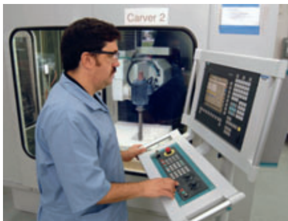
The five-axis milling robot designed by Bornemann uses the Sinumerik 840D CNC to allow versatile carving/milling operations
