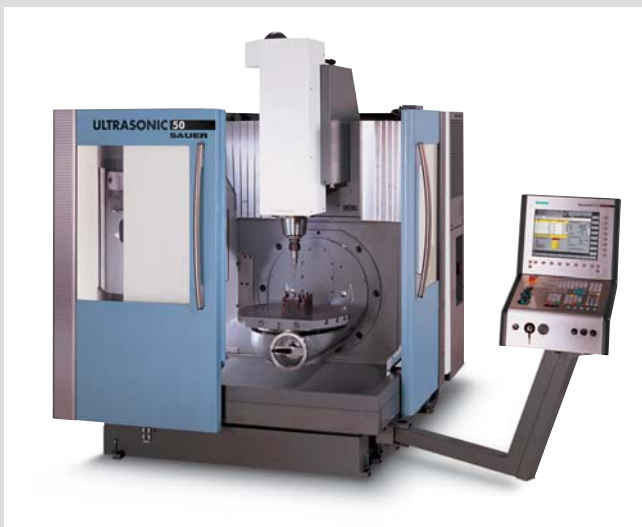
ULTRASONIC 50 from DMG, with machine travel (XYZ) of 500mm x 450mm x 400mm, features an HSK 63-S tool fitting that permits ultrasonic and conventional milling on a single three-axis machine.
