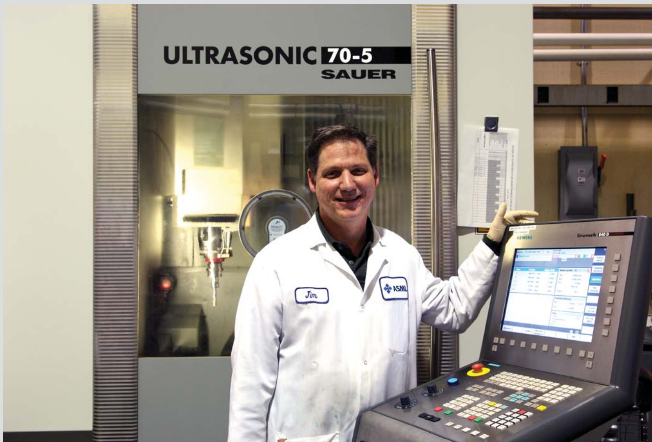
Jim Verrico, ASML Optics employee, operates the DMG 70-5. ASML produces various glass composite parts, especially from Zerodur, material with an extremely low coefficient of thermal expansion and outstanding 3D homogeneity. Parts are used by ASML parent company in The Netherlands in the building of various semiconductor, optic, medical and other equipment.
