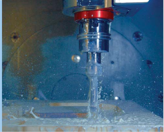
Zerodur block shown before and during ultrasonic glass machining process. Zerodur® is a registered trademark of Schott AG in Germany
