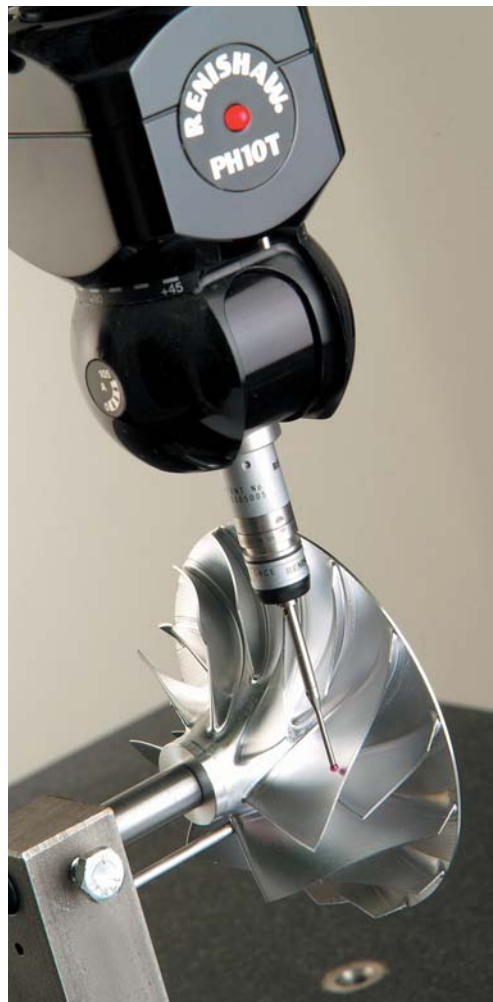
Left: Touch probe validating dimensions on the finished product.
