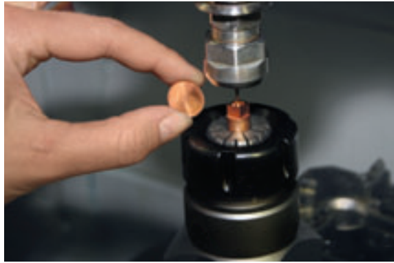
Technoplast achieves maximum precision to less than 5 micrometers and a perfect surface finish thanks to the HSC 20 milling machine and Sinumerik 840D
