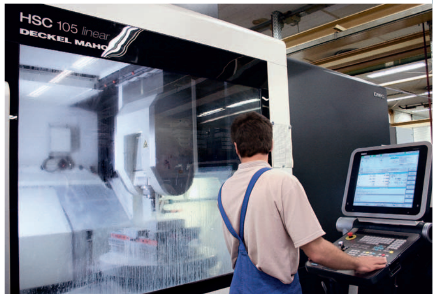
The five-axis HSC 105 linear milling center with Sinumerik 840D sl is perfect for high-precision tasks and is also very easy to operate
