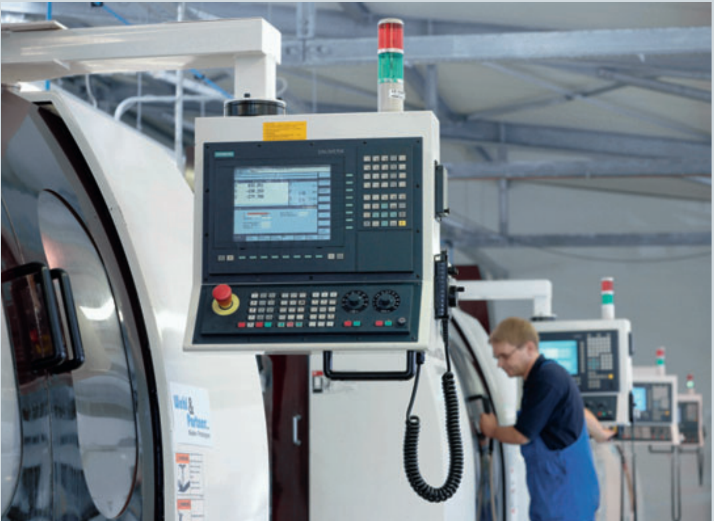
A supplier, a control system manufacturer: Wehl & Partner relies almost exclusively on CNC machining centers with Sinumerik 810D from Siemens
