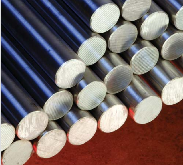
The machines used at CNC Industries produce high-precision medical instruments mostly from heat-treated 17-4 ph stainless steel, a material of superior hardness, strength and corrosion-resistance, therefore challenging to machine.
