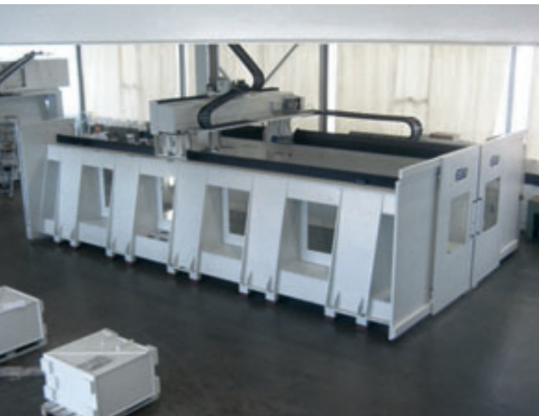
The HSC five-axis milling center for large volume aluminum or CFK parts can also process titanium and steel
