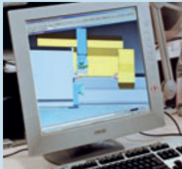
CNC machining programs are simulated offline as standard, in order to prevent errors and collisions right from the start
