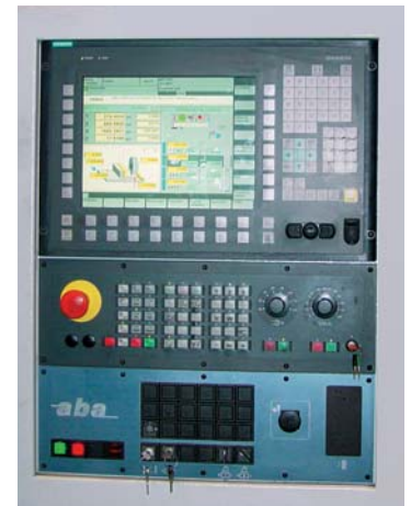
Above: The SINUMERIK 840D CNC and SIMATIC S7 PLC control package replaced three processors and independent operating systems on the customer's previous machine used for creep feed grinding of undercarriage links on a giant earthmover.
