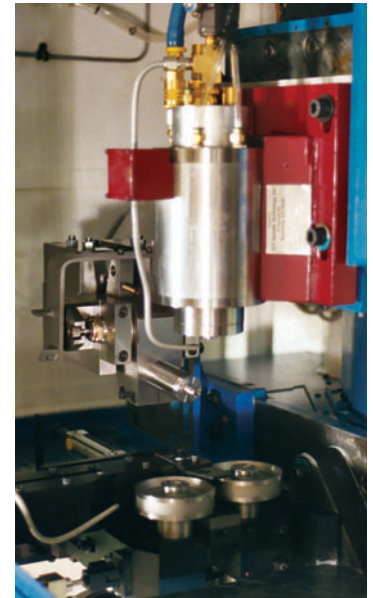
Above: The dresser and grinder spindles on the Heald machine run at High RPMs, controlled by the new CNC onboard. Eaton engineers report substantial improvements in the productivity of the machine, following the retrofit.
