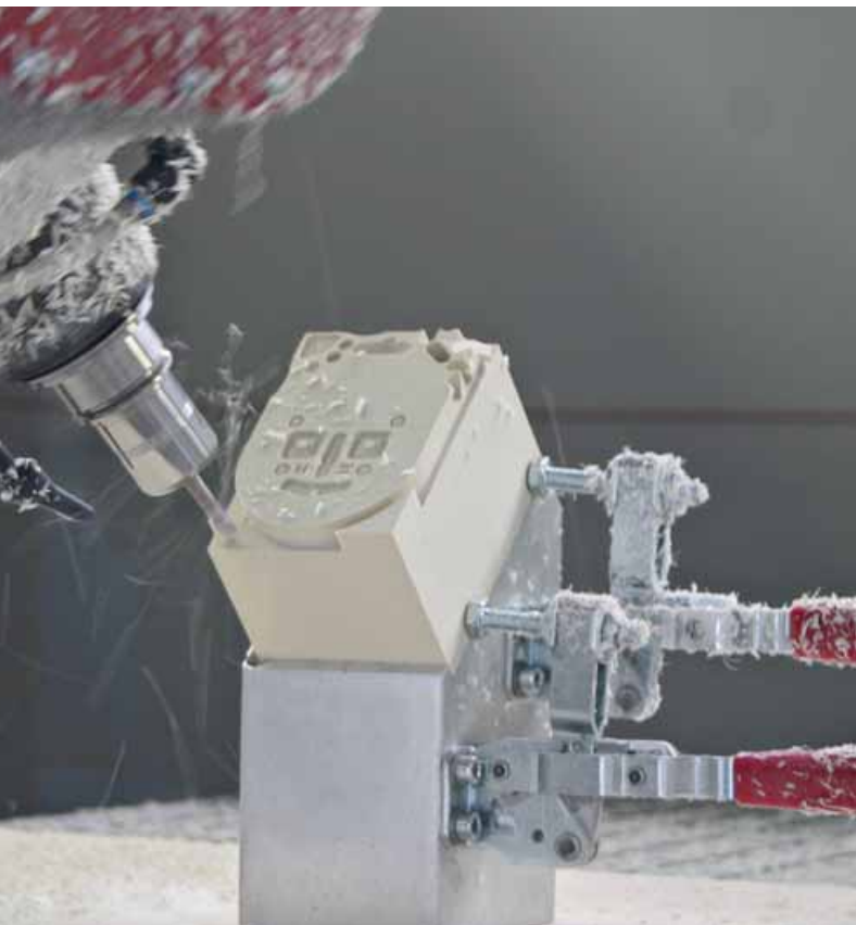
The machining center achieves an accuracy of 0.05 millimeters at the tool tip
